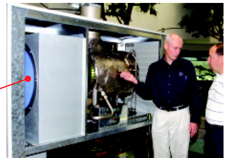
The blue Donaldson PowerCore air filter is on the front of this Capstone Microturbine unit.
